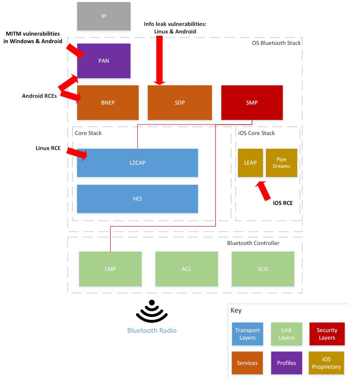
Basic blocks in the Bluetooth stack, indicating the location of various vulnerabilities
